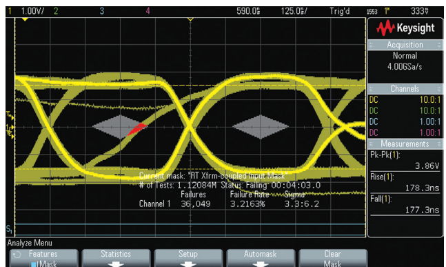
Figure 8: MIL-STD 1553 BC to RT xfrm-coupled input mask test reveals a shifted bit that violates the pass/fail mask.
